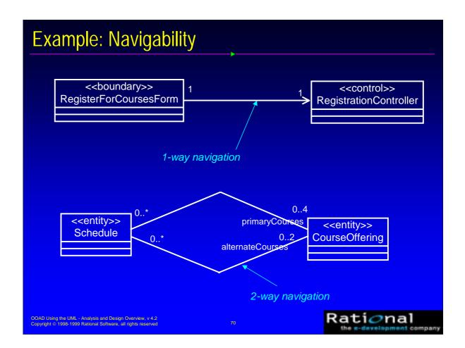
The top part of the above diagram demonstrates one-way navigation: A RegisterForCoursesForm invokes a single RegistrationController that will process the registration for the current Student (the Student that is building the current Schedule). The RegistrationController will never need to communicate directly to the RegisterForCoursesForm.
