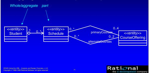
Aggregation is a stronger form of association which is used to model a whole-part relationship between model elements. The whole/aggregate has an aggregation association to the its constituent parts. A hollow diamond is attached to the end of an association path on the side of the aggregate (the whole) to indicate aggregation.
