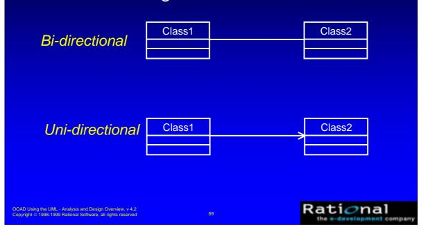
The navigability property on a role indicates that it is possible to navigate from an associating class to the target class using the association.
