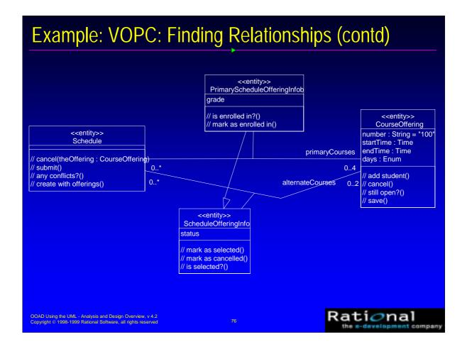
The above are the remaining classes from the Register for Courses VOPC. The complete VOPC was too big to fit on a single slide, so some of the classes are shown above and the remaining were shown on the previous slide.
