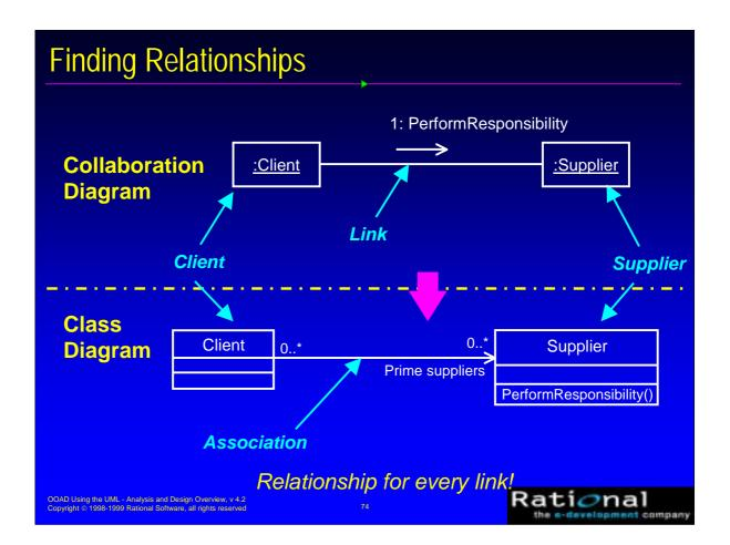
To find relationships, start studying the links in the collaboration diagrams. Links between classes indicate that objects of the two classes need to communicate with one another to perform the use case. Thus, an association or an aggregation is needed between the associated classes (the difference between these relationship types and when to use which was discussed earlier).
