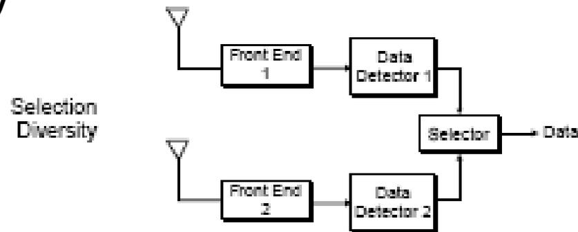
$$\bar{\gamma}_{\Sigma} = \int_0^{\infty} \mathcal{P}_{\gamma_{\Sigma}}(\gamma) d\gamma = \int_0^{\infty} \frac{\gamma^M}{\bar{\gamma}} [1 - e^{-\gamma/\bar{\gamma}}]^{M-1} e^{-\gamma/\bar{\gamma}}$$
