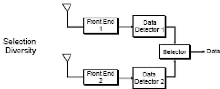
$$p(\gamma_i < \gamma) = 1 - e^{-\gamma/\bar{\gamma}_i}$$
